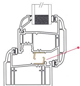
STAY GUARD use No1 for 17mm stack height on both Sash & Frame.
